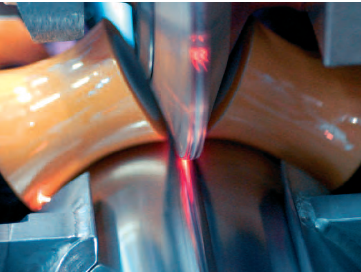
WELDING A MASHED CANBODY SEAM
