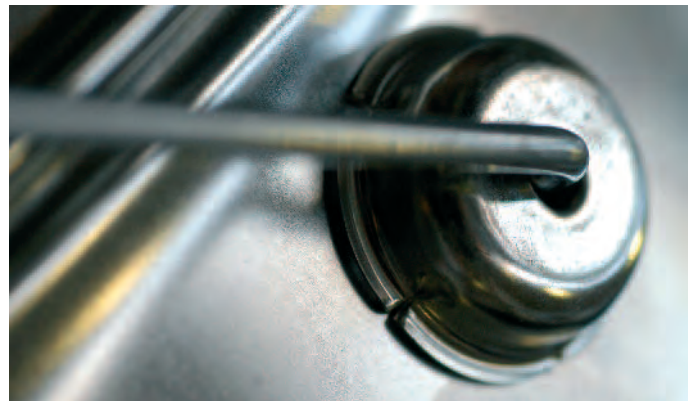
WELDING THE EAR TO THE CANBODY
