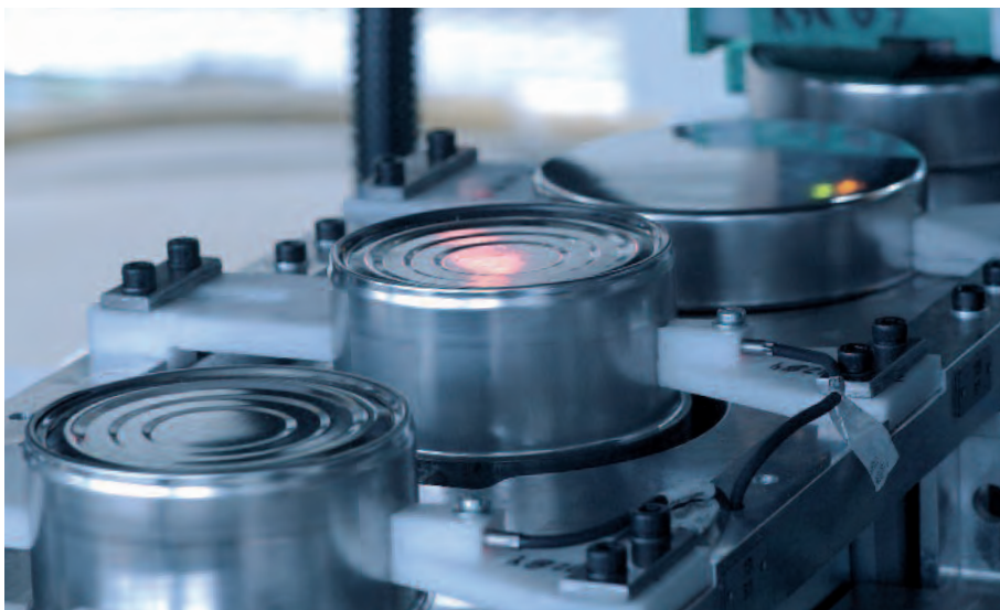
FINAL FORMING AND TRIMMING OF CANS
